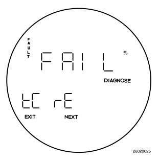
Figure 6-6. Fault 2, Reversed Thermocouple
